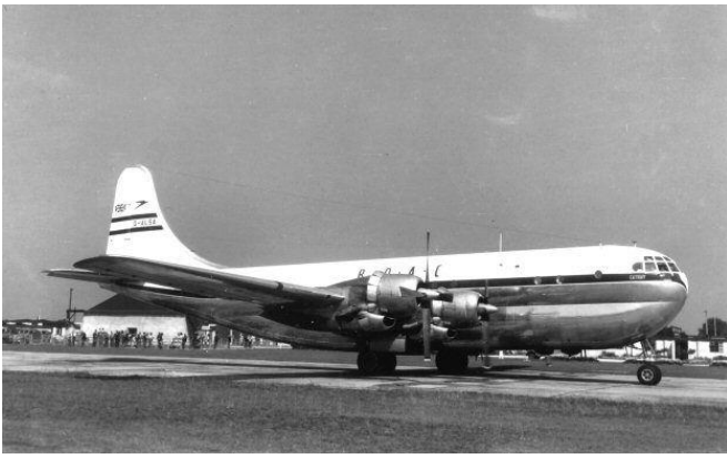
Left; G-ALSA, Cathay, one of the Stratocruisers originally ordered by SILA (SAS) was delivered to Heathrow on 12 October 1949. The SILA aircraft had circular windows on both decks and central galleys.
