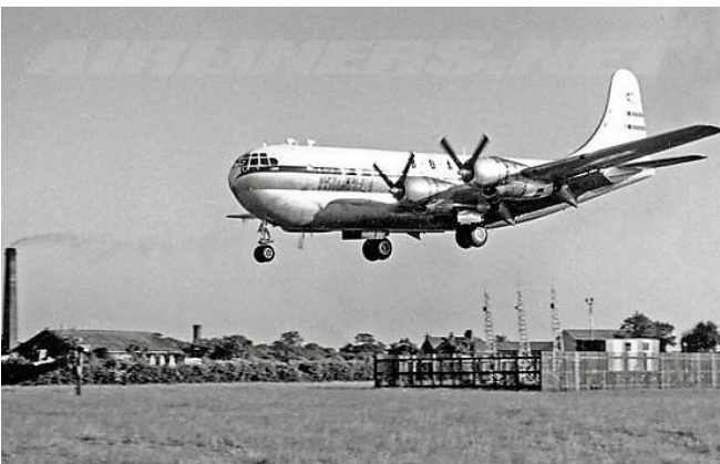
Above Left; Showing a nose-wheel low, massive flaps fully extended, final approach this BOAC Stratocruiser is about to pass the foul-smelling animal products factory in the background. (Airliners photo). Above Right; G-ANUM, formerly Pan Am N1027V, was the first Stratocruiser from the BOAC fleet to be sold, on 5 August 1958. It was re-sold by the Babb Company to Transocean Air lines and reverted initially to its previous registration N1027V and was then re-registered N401Q. Sold at auction in 1960, it was subsequently scrapped. (Airliners photo)
