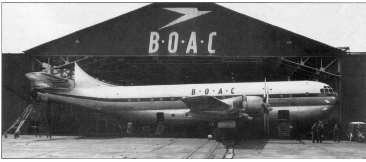
Left; The fin on this aircraft is not damaged. In fact, the fin has been folded, as it was designed to allow Stratocruisers such as this to be manoeuvred into or out of a hangar.
