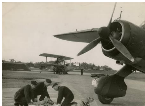
The Walrus was a British amphibious biplane reconnaissance aircraft designed by R. J. Mitchell and first flown in 1933. Used as a fleet spotter for catapulting from RN ships (Left) the Walrus was later employed in Air Sea Rescue (Right with Lysander in the foreground). On several occasions Walrus ASRs taxied across the Channel with rescued Allied airmen on board because the sea was too rough to take-off! (Interestingly the Walrus was originally known as the Supermarine Seagull V)
