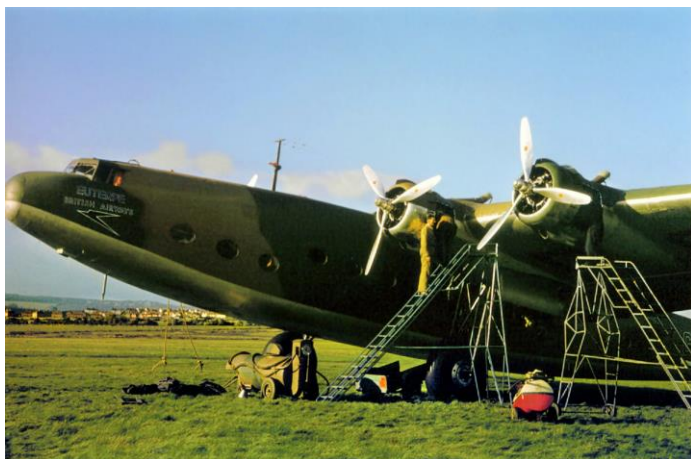
Above Left; A survivor from pre-WWII operation by Imperial Airways, an Armstrong Whitworth Ensign airliner undergoes maintenance, probably at Whitchurch, Bristol, the British Overseas Airway's temporary dispersed base. Camouflaged G-ADTA Euryalus wears British Airways titling, a Speedbird logo and has Wright Cyclone engines fitted. It had a short wartime life, however, as it crash landed at Lympne on 23 May 1940 after escaping from France. It was then transported to Hamble, where it was original built, and written off and cannibalised to repair G-ADSU Euterpe .
