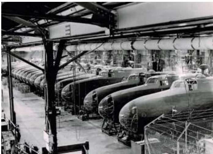
Above Left; A WWII view of the Aldenham Works, with a selection of workers cars parked nearby. These would have been for management with a need for petrol coupons. Above Right; Aldenham – the assembly line for aircraft centre sections, with outer skins being applied. Below Left; Halifax nose sections being fitted out internally at Aldenham
