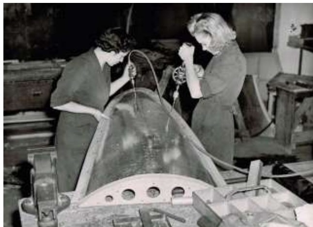
Above Left; Park Royal Coachworks in Abbey Road, Park Royal. Above Right; Two young ladies assemble a Halifax wingtip, using pneumatic and hand drills. Surely the workpiece would normally be supported in a jig?
