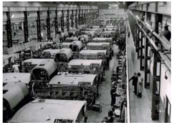
Above Left; A WWII view of the Aldenham Works, with a selection of workers cars parked nearby. These would have been for management with a need for petrol coupons. Above Right; Aldenham – the assembly line for aircraft centre sections, with outer skins being applied. Below Left; Halifax nose sections being fitted out internally at Aldenham
