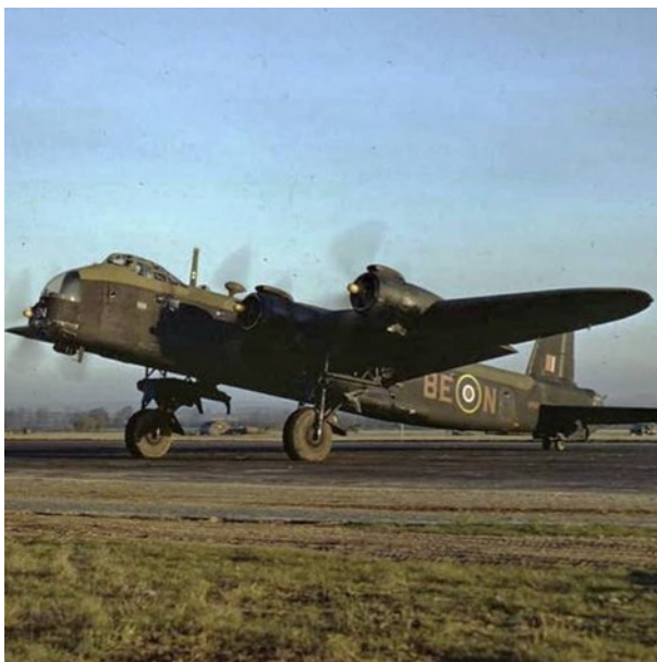
Photo Left; A glider towing Short Stirling, - note the glazed nose position in place of the front turret.
