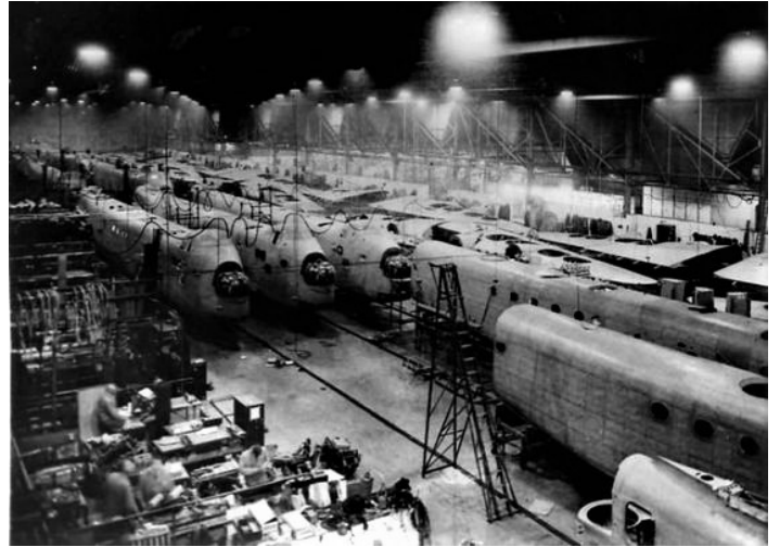
Above Left; Mass production of Stirlings underway. Above Right; A further photo of Stirling production. Note the cabin windows that were thoughtfully provided for when aircraft were used in their secondary passenger/ trooping role.
