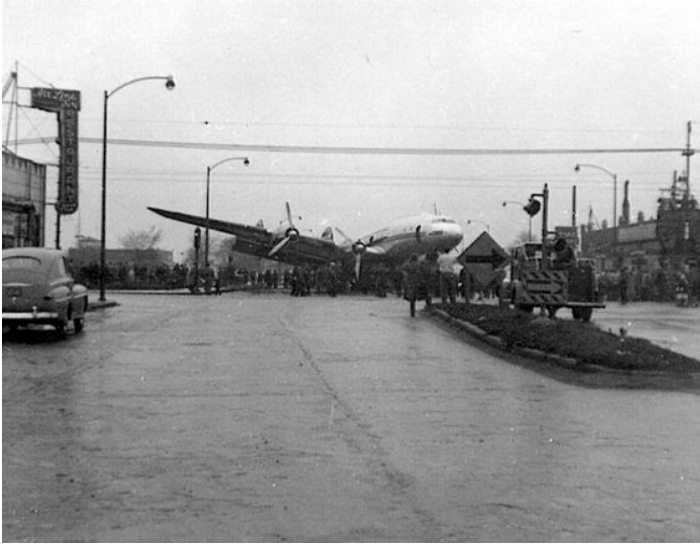
Above Left; On 18 December 1949 N86501 landed 'long' at Chicago Midway (3,200 feet down Runway 13R with 2,530 feet left) and then continued for a further 875 feet to arrive on Cicero Avenue, only stopping after striking a stone monument and the Acme Bar and Grill.
