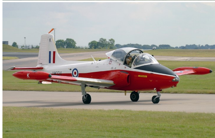
Above Left; The BAC Jet Provost T.5 was an improved design distinguishable by a different nose shape to earlier variants. BAC modified many T.5 aircraft with improved avionics and a rough grey coating on the wing to break up the smooth airflow and give the trainee pilot an early indication of the onset of a stall. XW370 was one such T.5A. Above Right; Wing tip tanks were not a regular feature of the T.5, unlike XW324 that retained them in to preservation as G-BWSG.
