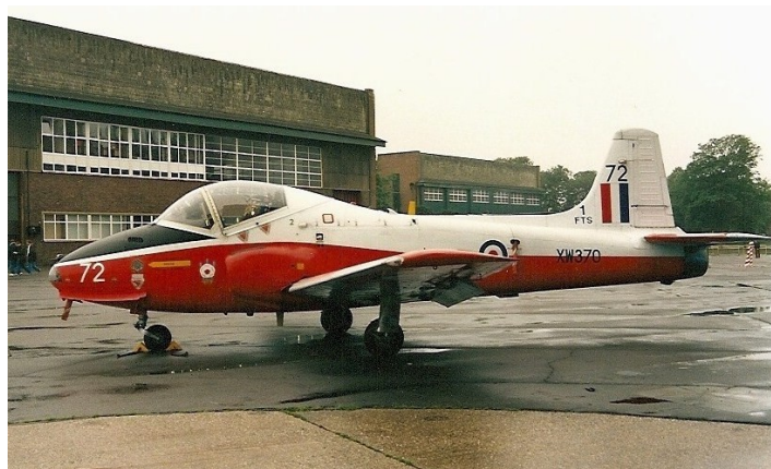
Above Left; The BAC Jet Provost T.5 was an improved design distinguishable by a different nose shape to earlier variants. BAC modified many T.5 aircraft with improved avionics and a rough grey coating on the wing to break up the smooth airflow and give the trainee pilot an early indication of the onset of a stall. XW370 was one such T.5A. Above Right; Wing tip tanks were not a regular feature of the T.5, unlike XW324 that retained them in to preservation as G-BWSG.
