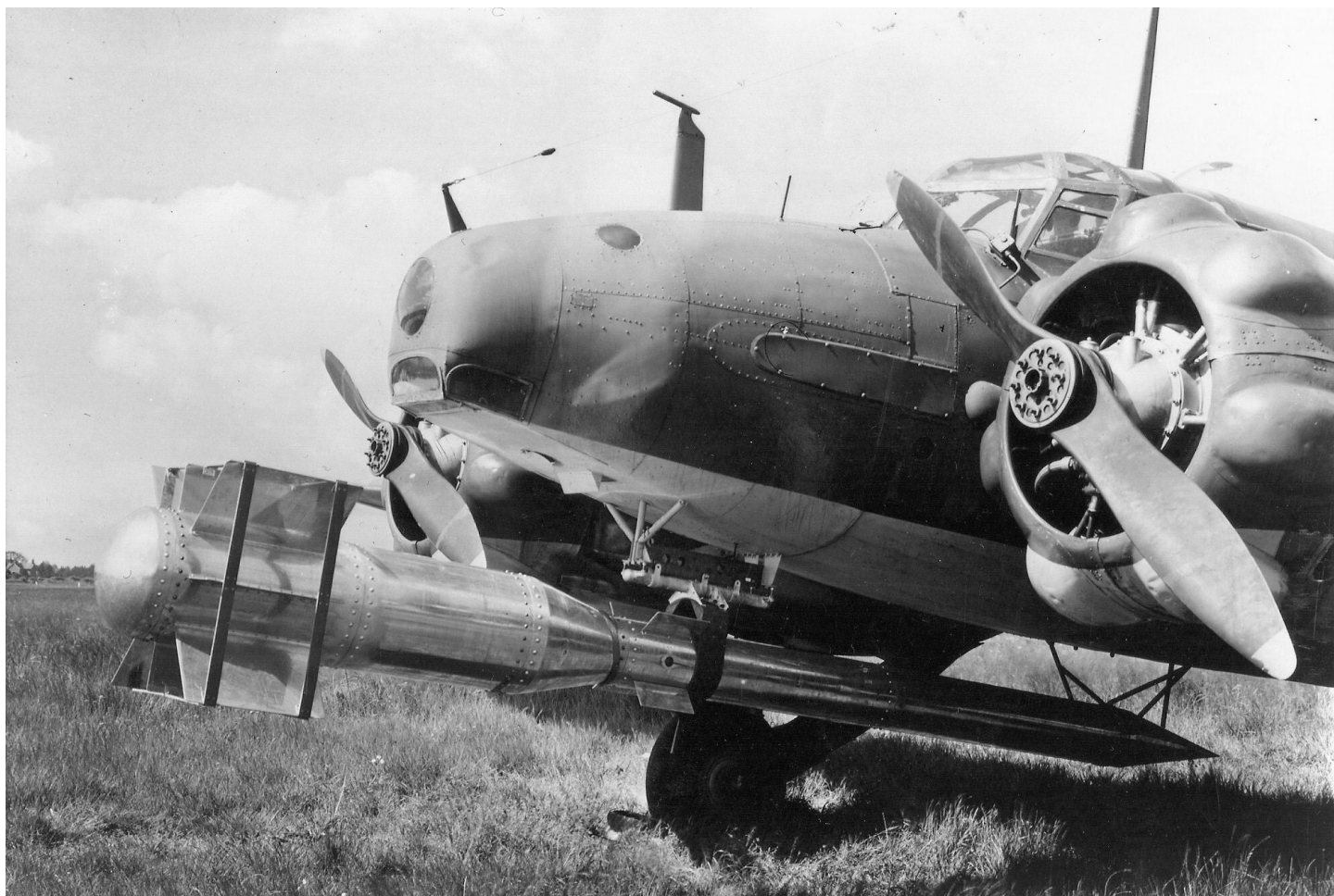
Above; An Anson of the Naval Air Radio Installation Unit at RAF Christchurch lent an aircraft to the Signal Research Establishment in May 1945, in order to test the telemetry of the signals by flying down the control 'beam'. It was attached under the Anson, on a support bracket used for the ASH radar pod, as used by Naval aircraft, such as the Firefly NF.
