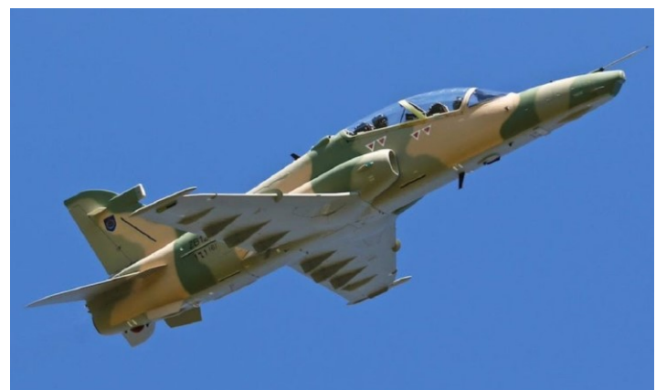
Above Left; the first of 12 Eurofighter Typhoons ordered by the RAFO with a combination of dual and single cockpit types. Above Right; The Hawk 100 series was designed to be even more suited to combat duties and advanced weapons training. It had a radar warning receiver (RWR), forward looking infrared (FLIR), chaff and flare dispenser, 'hands on throttle and stick' HOTAS controls, multi-function displays (MFD) and a head-up display (HUD), whilst the 'combat wing' included wingtip launch rails for air-to-air missiles. In the RAFO, desert camo colours are used for low level ops.
