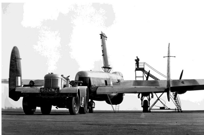
Above Left: RF342 with SE210 Caravelle section on 16 th Apr 1959. Above Right; a David Brown tractor ready to tow Lincoln RF342 at Luton. Note the aerofoil mounted on top of the fuselage ready for testing.
