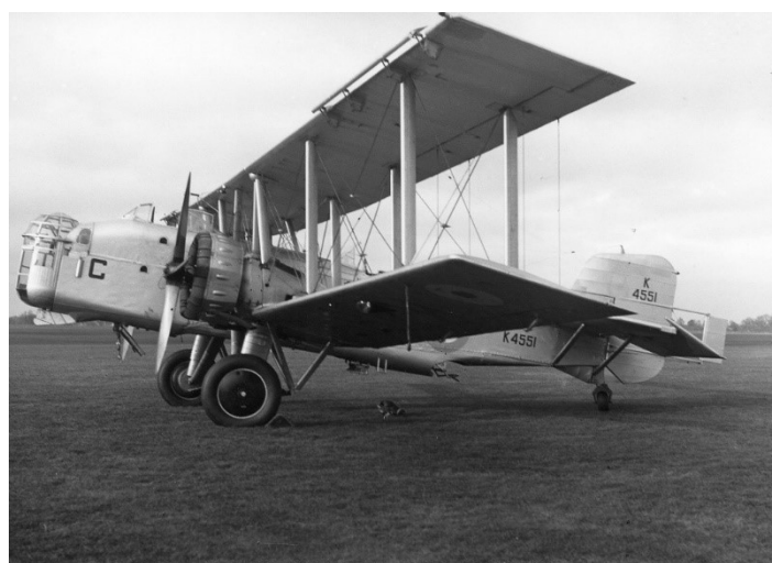
Above Left; DH.60 Gipsy Moth, K1200, in India in 1930s. Above Right; Boulton & Paul P.75 Overstrand, K4551 'C' of 101 Sqn, at RAF Bicester in 1936. The Overstrand was the first RAF aircraft type to have a power operated turret.
